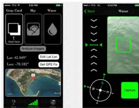
Fig. 2 The HydroColor user interface showing the prompts for the three images: grey card, sky, and water (left). On selecting the image, the screen changes to display the inclinometer and compass to guide the user to the correct smartphone angle to capture the image (right). When the green elements of the compass and inclinometer are properly aligned with the green triangles, the capture button turns green enabling the photo to be taken.
