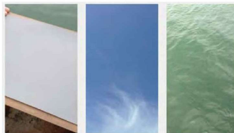
Fig. 1 Example images of the 18% photographer’s grey card (left), the sky (middle), and the water surface (right) collected by a HydroColor user for calculating the remote sensing reflectance ( http://miscilab.umeoce.maine.edu/research/HydroColor.php ).
